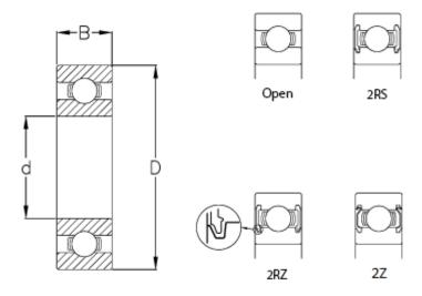
B = 16 Ball grade = 5 C (KN) = 22.1 C0 = 14.6 d = 45 D = 75 Max rpm. = 16000 Type = 6009
